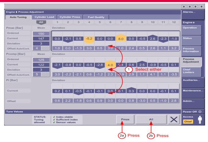
Depending on selected panel the button text (2a) will change – Pmax, Pcomp or Pi Select the All button (2b) to simultaneously balance Pmax, Pcomp and Pi.
